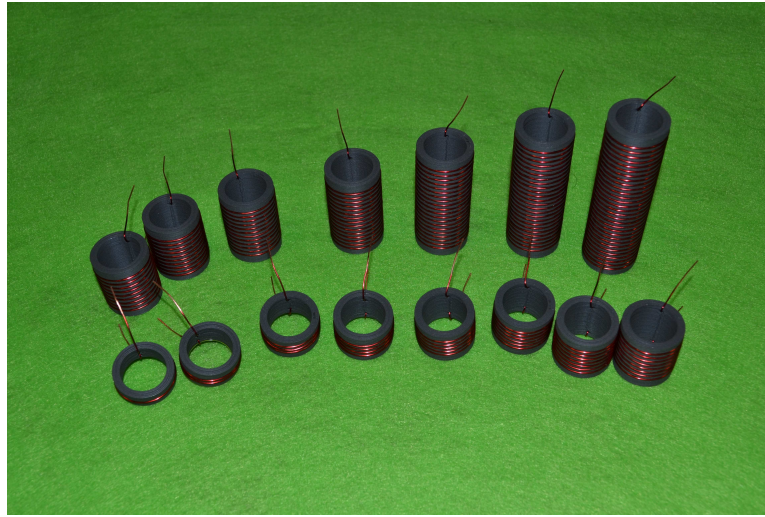
Figure 13: Iron composite PLA coils, 1 to 30 turns
