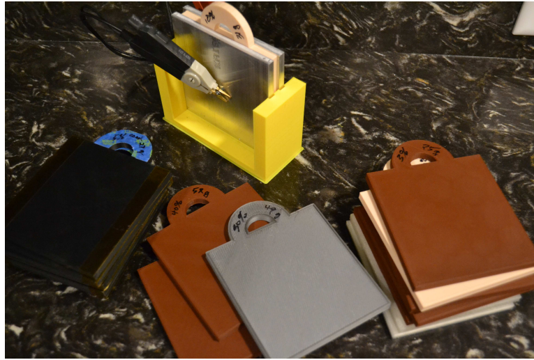
Figure 39: Permittivity test panels.
