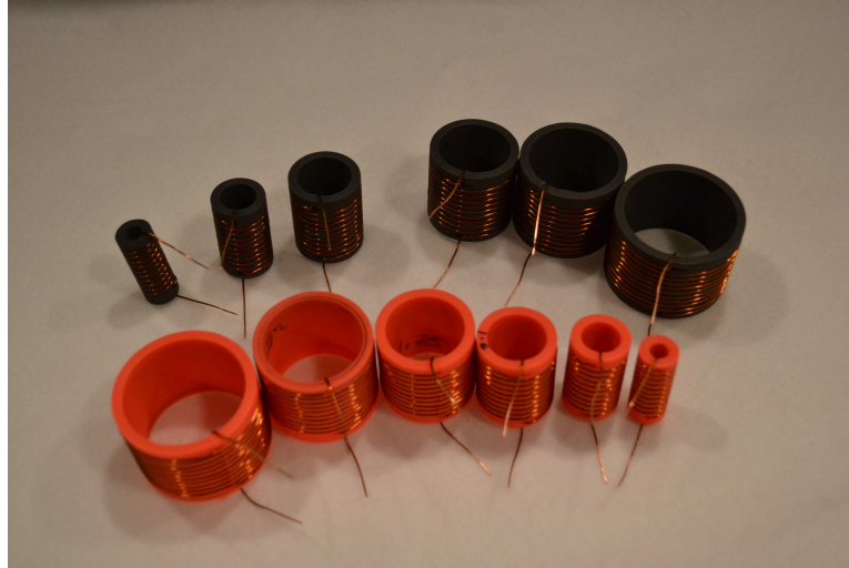
Figure 19: 10 turns, .1 spacing, diameter 0.5 to 1.75", #22 wire. Plain PLA front, Iron Composite in the back.
