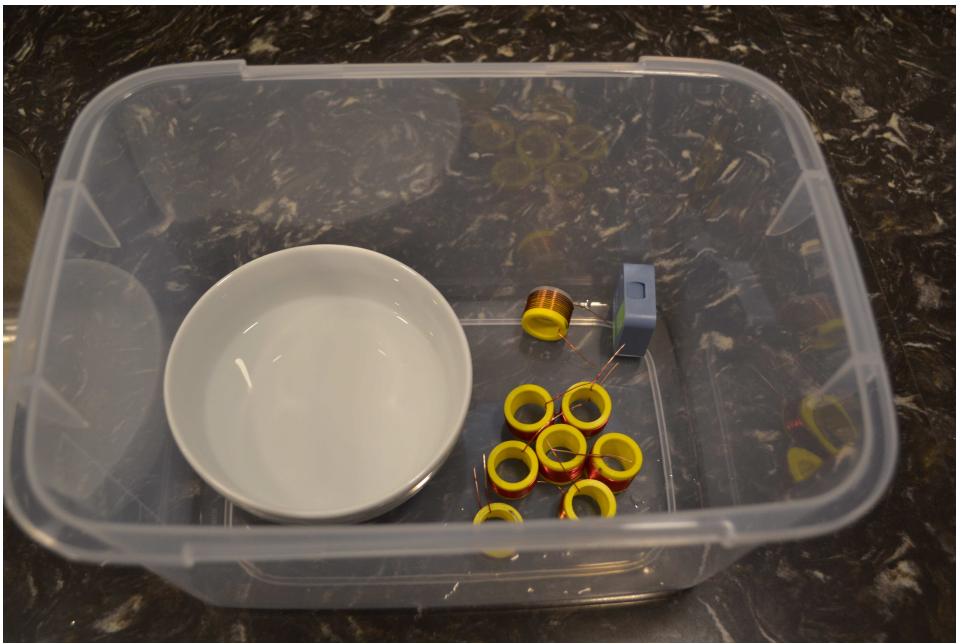
Figure 48: High humidity chamber.
